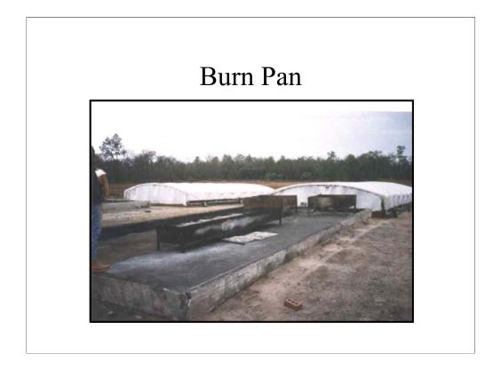
Note the covers in the background which can be rolled over the units to prevent accumulation of precipitation.
